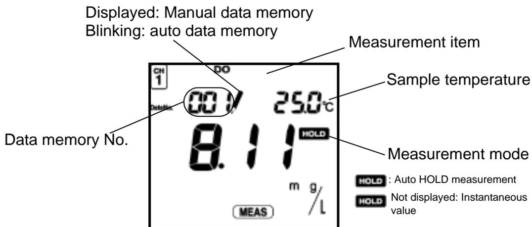
Select and load the desired memory data item using the
