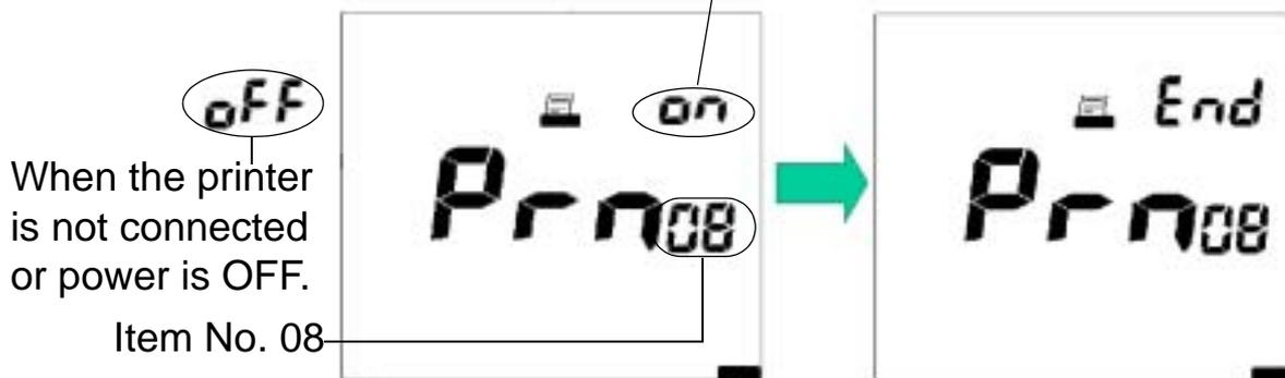
2. Press the MODE key to return to the first item in the maintenance modes, LCD check.
