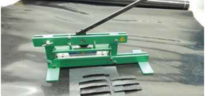
Blank in uniform size, quickly produced with the Coupon Cutter.
