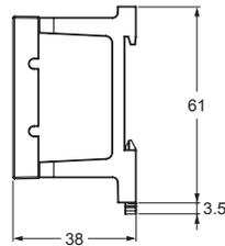
This Adapter is used to mount the E5CC to a DIN Track.
