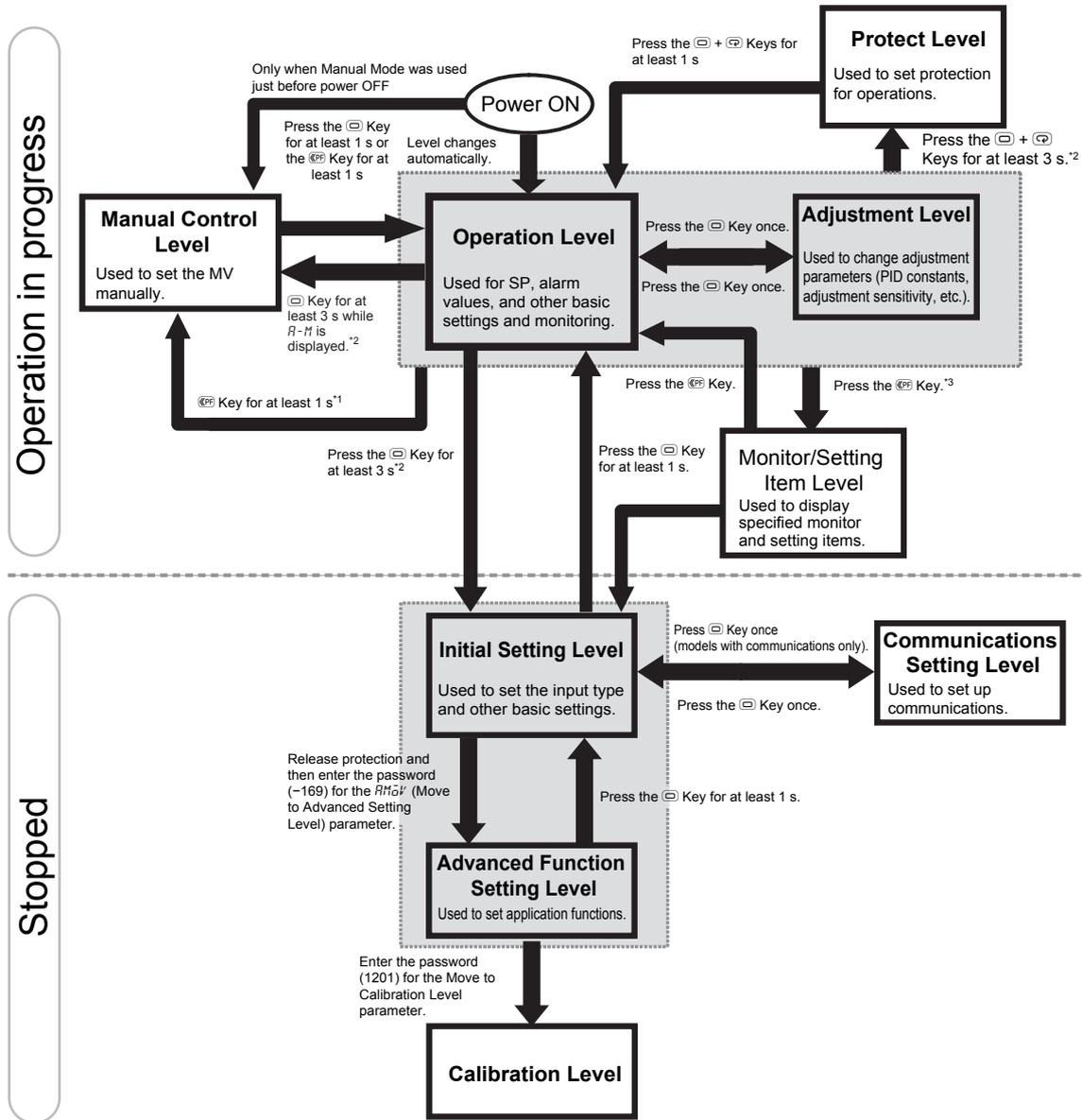
\*1 To use a key procedure to move to Manual Control Level, set the Auto/Manual Select Addition parameter to ON and set the PF Setting parameter to  $R-M$  (Auto/Manual).
