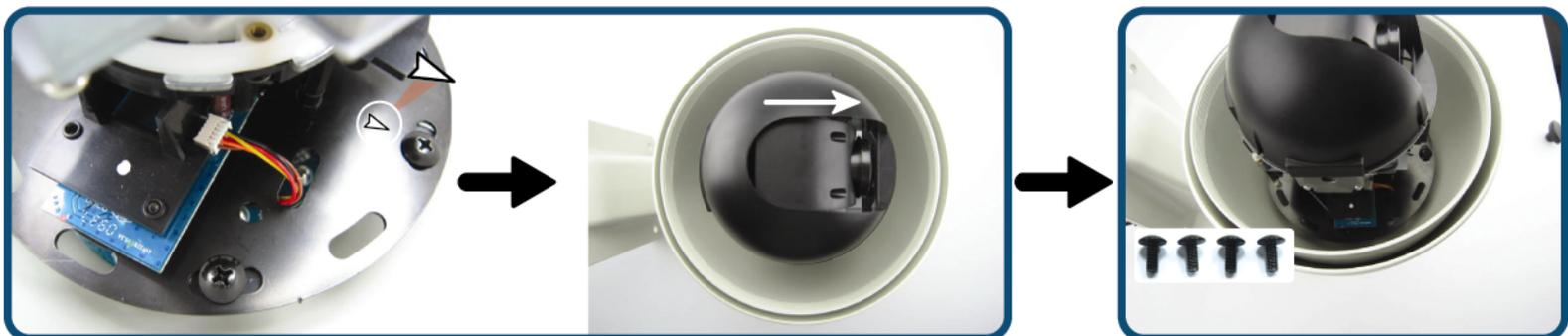
Find the mark “>” on the iron plate of the camera module, and rotate the plate with the mark “>” to face the direction opposite to the bracket.
