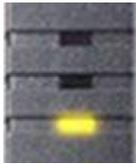
When the Main Unit operates in normal mode, the yellow LED is flashing every second.
