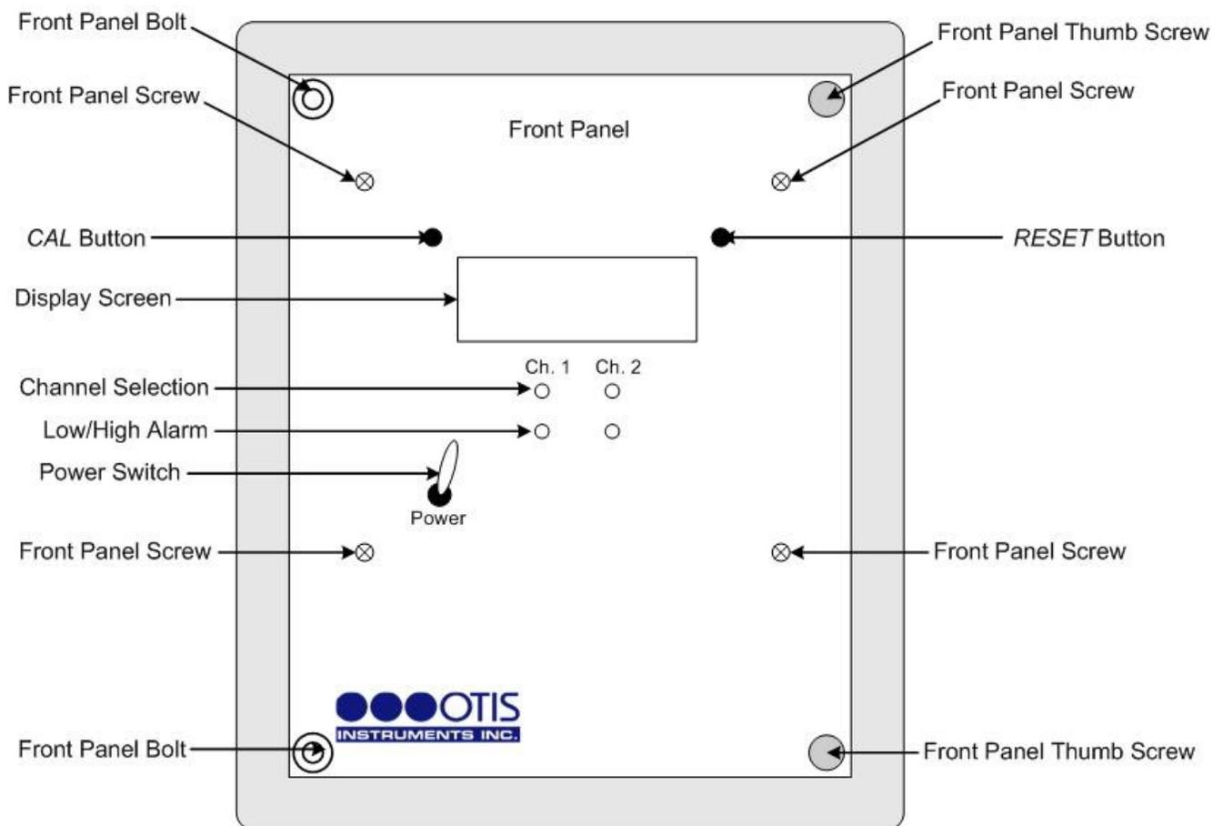
4. Flip the Power Switch upward.
