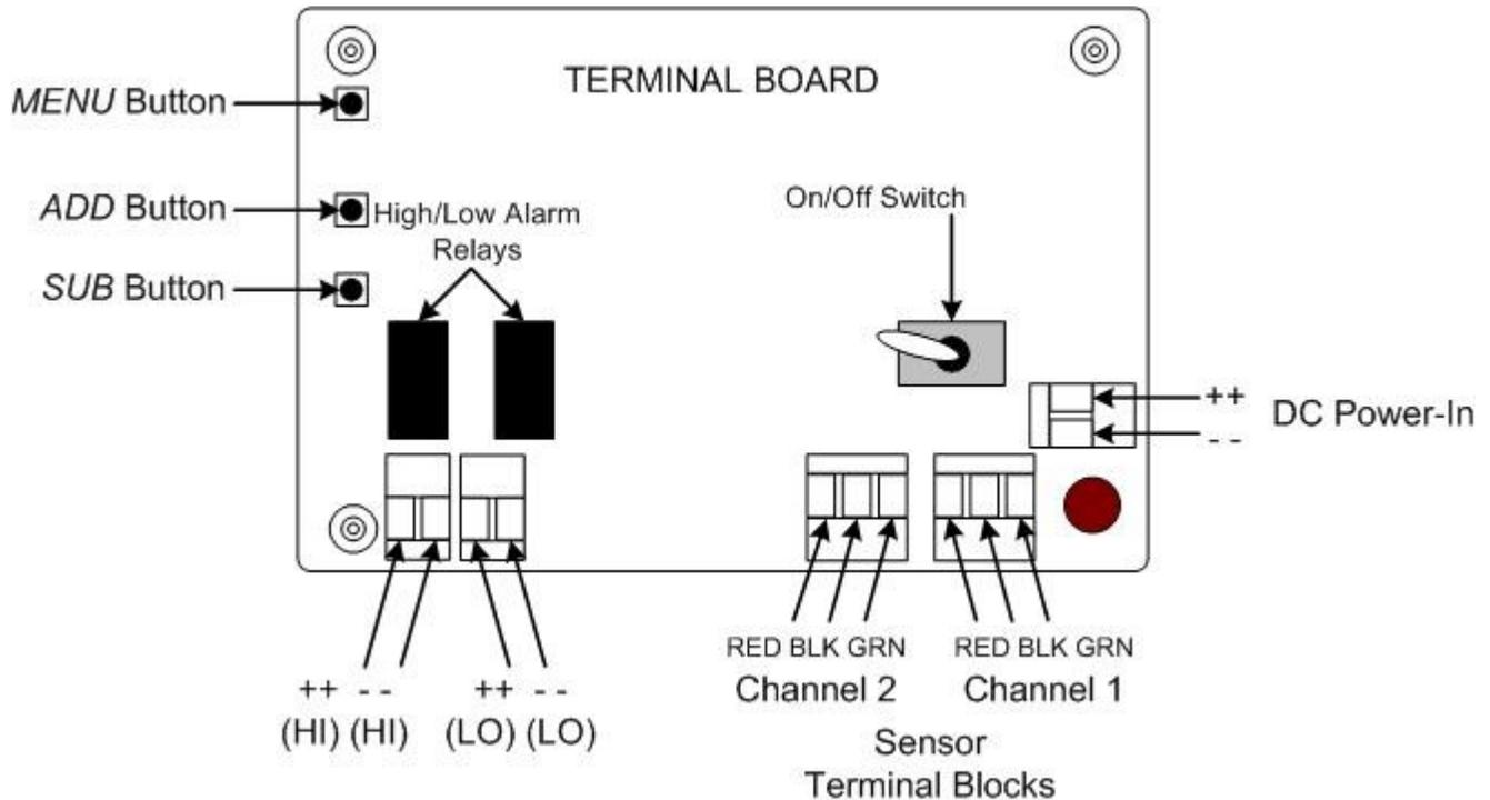
2. Wire the first sensor assembly to the Channel 1 Sensor Terminal Block as follows:
