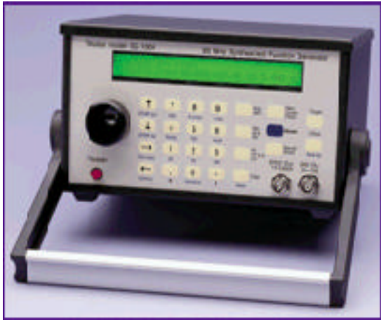
Figure AA-10. Telulex Model SG-100/A otherwise known as the BNC Model 625A signal generator.
