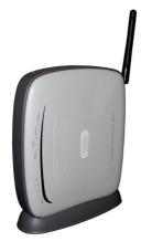
The 802.11g Router is a small desktop router that sits between your local Ethernet network and a remote network (e.g., the Internet). The 802.11g Router contains an WAN port connecting to an external ADSL/Cable modem, a DMZ port, a four-port 10/100Mbps Ethernet switch for connection to PCs on your local wired network, and a wireless interface for connection to your local wireless network (supporting a data rate of up to 54 Mbps).
