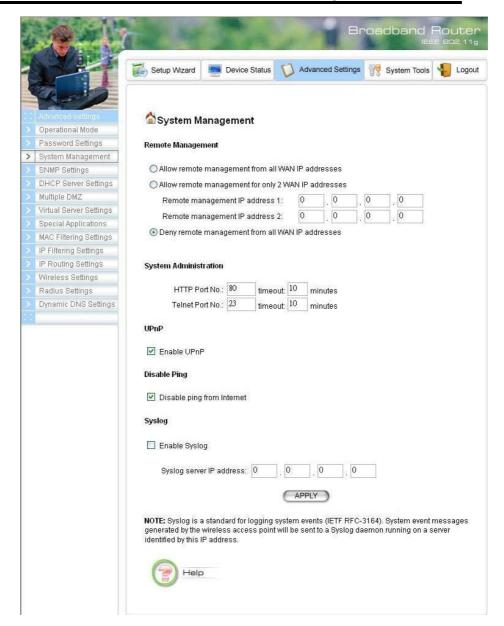
**NOTE:** Syslog is a standard for logging system events (IETF RFC-3164). System event messages generated by the Wireless router will be sent to a Syslog daemon running on a server identified by this IP address.
