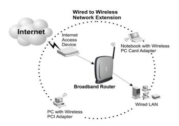
**Making WLAN Connections**
