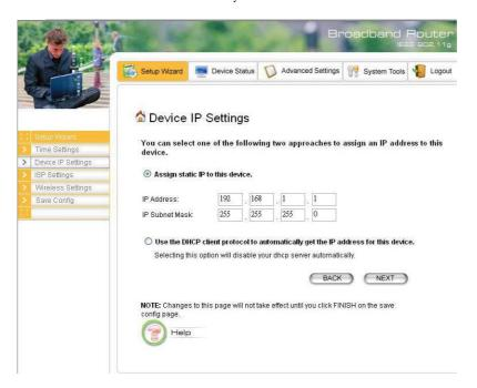
If you choose to assign a static IP address manually, check the button that says, "Assign static IP to this device" and then fill in the following fields
