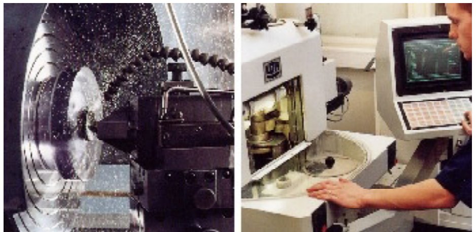
Figure 22.4 LEFT: Diamond turning machine; RIGHT: Lens polishing
