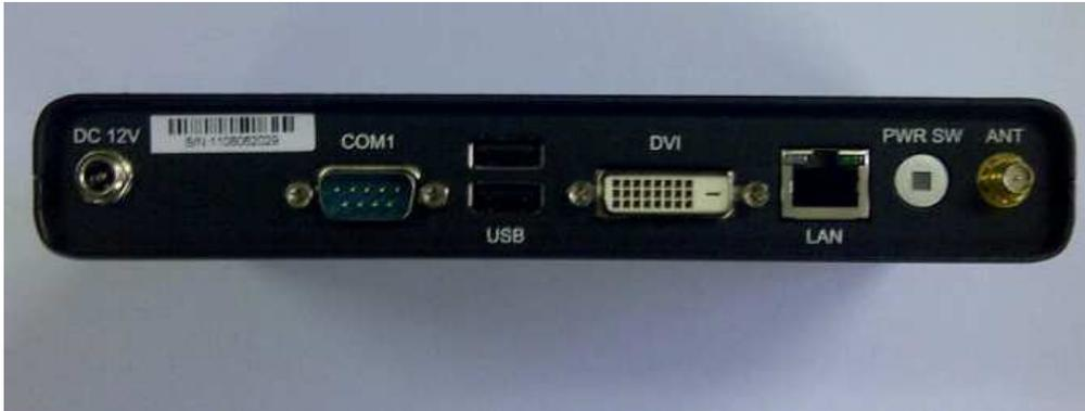
Figure 2: The back panel of the VR-100A
