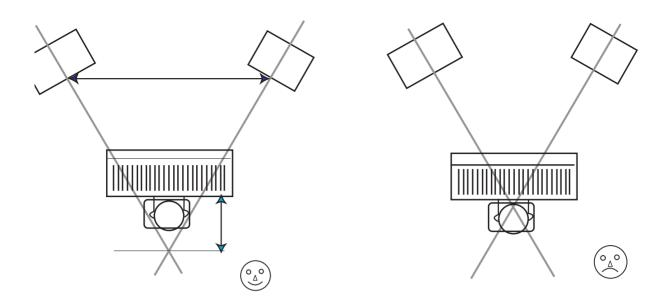
The height of mounting the speaker is equally as important. The correct height should result in the axis being at ear level when the engineer is sitting in his normal position at the console.
