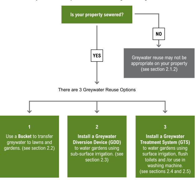
Each reuse option has different permitted end-uses and approval requirements. Tables 1 and 2 show how greywater can be reused depending on the treatment method and depending on whether it is for a single residence or a multi-dwelling/commercial premises
