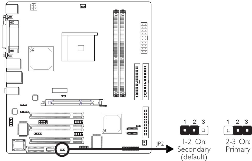
CNR cards are defined as primary and secondary. Set this jumper according to the type (primary or secondary) of CNR card installed in the CNR slot.
