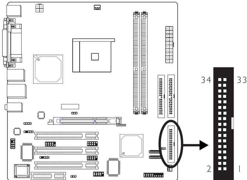
The system board is equipped with a shrouded floppy disk drive connector for connecting two standard floppy disk drives. To prevent improper floppy cable installation, the shrouded floppy disk header has a keying mechanism. The 34-pin connector on the floppy cable can be placed into the header only if pin 1 of the connector is aligned with pin 1 of the header.
