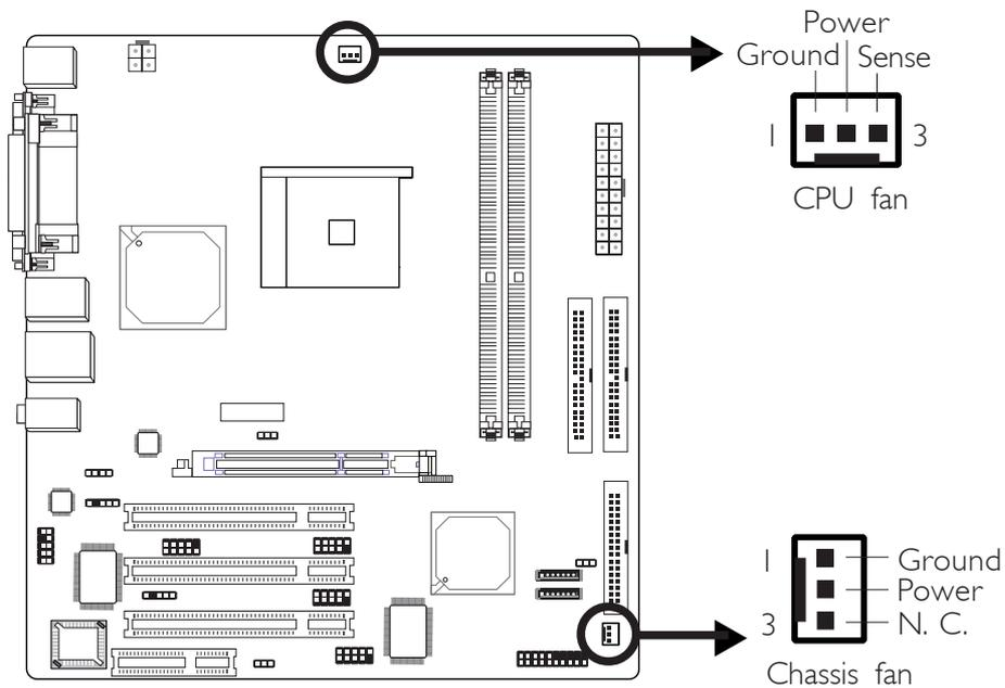
Connect the CPU fan's cable connector to the CPU fan connector (J20) on the system board. The chassis fan connector (J10) is used to connect an additional cooling fan. The cooling fans will provide adequate airflow throughout the chassis to prevent overheating the CPU and system board components.
