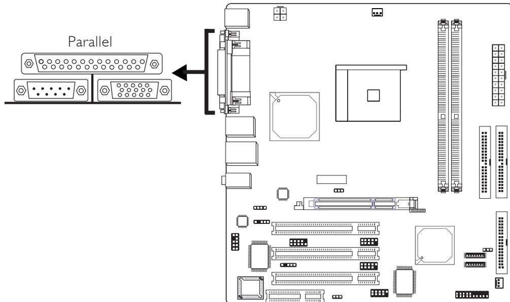
The system board has a standard parallel port (Burgundy) at location CN7 for interfacing your PC to a parallel printer. It supports SPP, ECP and EPP.
