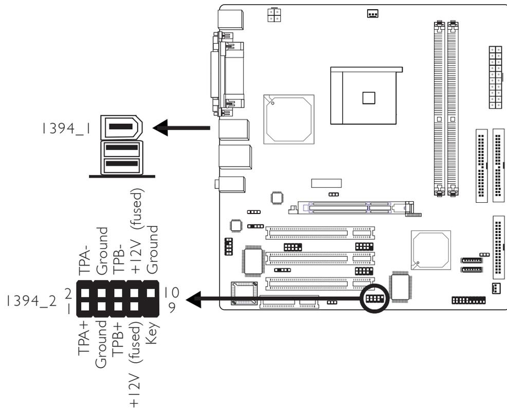
The system board is equipped with an onboard IEEE 1394 port at location CN6 (IEEE 1394\_1) of the system board.
