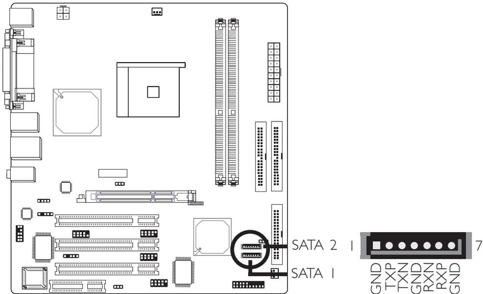
Connect one end of the Serial ATA cable to J15 (SATA 2) or J16 (SATA 1) and the other end to your serial ATA device.
