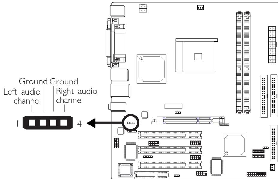
The CD-in (J2) connector is used to receive audio from a CD-ROM drive, TV tuner or MPEG card.
