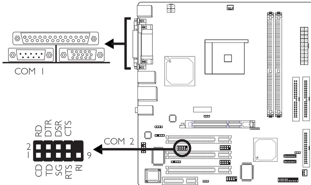
The system board is equipped with an onboard serial port (Teal/Turquoise) at location CN4 for COM 1. It is also equipped with a 9-pin connector at location J6 for COM 2.
