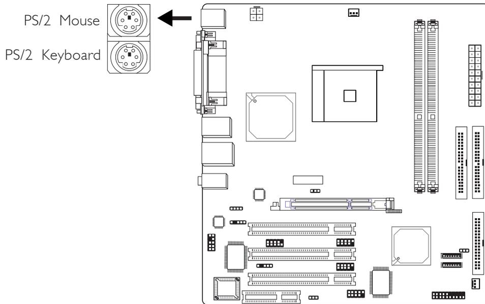
The system board is equipped with an onboard PS/2 mouse (Green) and PS/2 keyboard (Purple) ports - both at location CN1 of the system board. The PS/2 mouse port uses IRQ12. If a mouse is not connected to this port, the system will reserve IRQ12 for other expansion cards.
