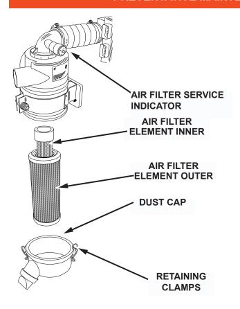
NOTE: The indicator may return to the nonviable position when the engine is shut off. To check, reset indicator and turn on the engine, if it locks in visible position again clean or change element.
