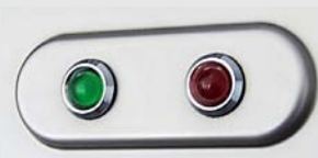
The coloured indicators make it easy to see whether the machine is working (red) or ready for loading or unloading of pots (green).
