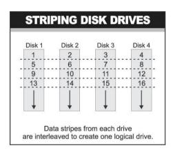
By striping the drives in the array with stripes large enough so that each record falls entirely within one stripe, most records can be evenly distributed across all drives. This keeps all drives in the array busy during heavy load situations. This situation allows all drives to work concurrently on different I/O operations, and thus maximize the number of simultaneous I/O operations that can be performed by the array.
