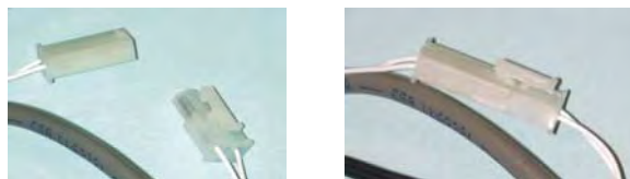
Figure A2.2. Switching hardware between SDI-12 and RS-232 modes.
