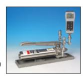
System F is an easy-to-use calibration system. The hydraulic pump makes it very easy to prime the system. The pump contains 75 in 3 / 1.23 I of liquid.
