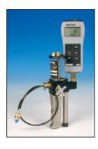
System C is an easy-to-use single hand-operated calibration system. No need for a flat surface (table) to operate the system. The system includes release valve and vernier valve for fine adjustment to enable safe and simple operation of the pump.
