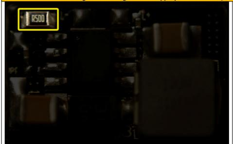
The yellow mark shows the place of the sense resistors. 0805 size package resistors is required.
