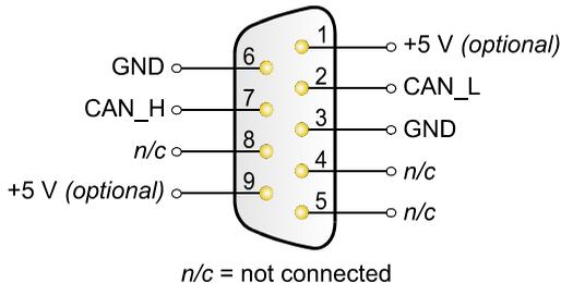
Figure 1: Pin assignment HS-CAN
