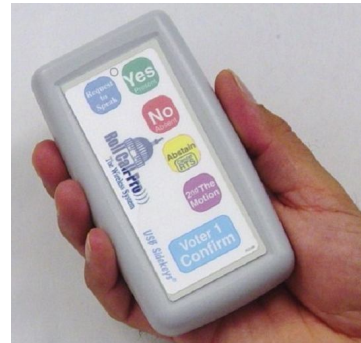
Figure 4-2. Wireless Member Keypad
