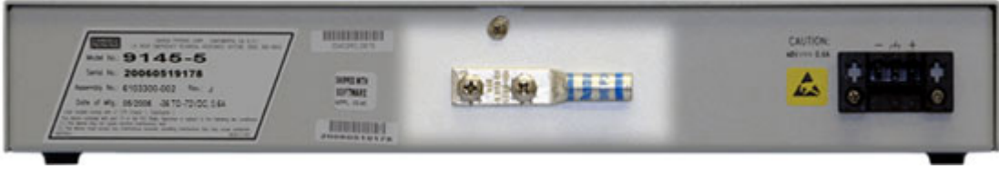
Figure 8 – Ground Lug Location
