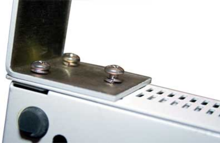
Figure 5 – Bracket Attachment Detail
