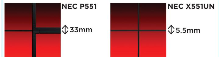
The X551UN's ultra-narrow bezel allows for a screen-to-screen distance between two neighboring displays of only 5.5mm, close to 450% improvement compared to its previously revolutionary 33mm P Series displays.
