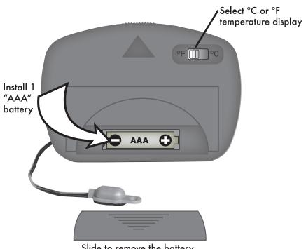
Slide to remove the battery compartment cover
