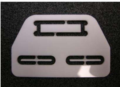
Example with two bridges in each curve to hold the inner part in place
