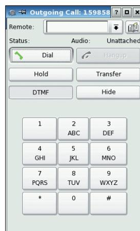
**Figure 5: KPhone makes life easy for newbies. You can produce DTMF tones at a push of a button, and use them to query an answering machine.**
