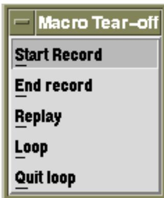
The macro facility allows the user to record a sequence of actions which can then be replayed so that series of repeated actions can be automated. On replay the actions involving interaction with the image e.g. one of the painting tools will wait until painting is confirmed before continuing.
