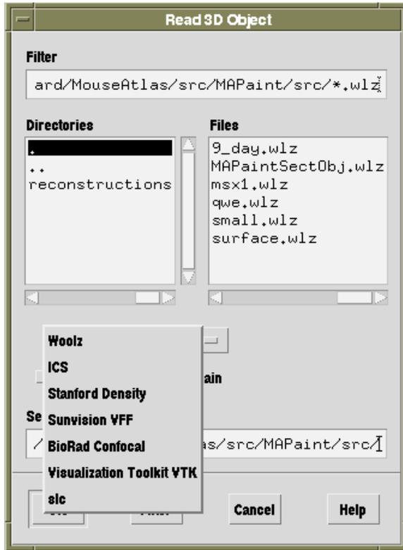
The choice menu below the directory and file windows allows the selection of other image formats. Selecting a format will automatically reset the filter for the default file extension. If the required file does not have this extension then it can still be input but to make the file visible in the file list change the filter line to read in all files by removing the .??? following the asterisk (\*) and pressing “return” or click the filter button.
