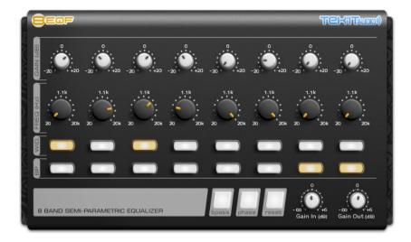
8eqf can be used in stereo or mono as an insert effect or as send/return effect.
