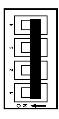
ALL 4 SWITCHES ARE JOINED TOGETHER VIA A BAR PLACED ACROSS THE TOP OF THE SWITCH. THIS IS A DETAIL VIEW OF THE 4-POSITION DIP SWITCH THAT HAS BEEN "GANGED"
