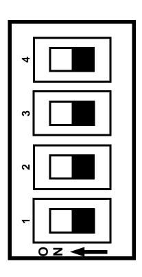
THIS IS A DETAIL VIEW OF THE GRAYHILL 4-POSITION DIP SWITCH USED ON THE TURBOTRACK CARD. PLEASE NOTE THE DIRECTION OF THE DIP SWITCH FOR THE "ON" POSITION. THE SWITCH MUST BE PUSHED TOWARD THE NUMERICAL INDICATOR (THE DIRECTION OF THE ARROW) TO BE IN THE "ON" POSITION.
