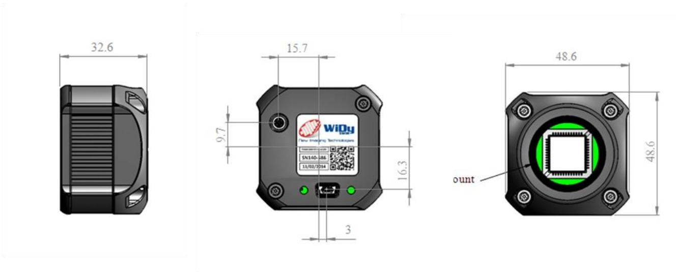
Figure 7 - WiDy 640U-S Dimensions (mm)
