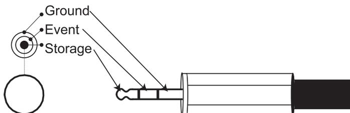
Connect signal leads inside the plug using the following diagram.
