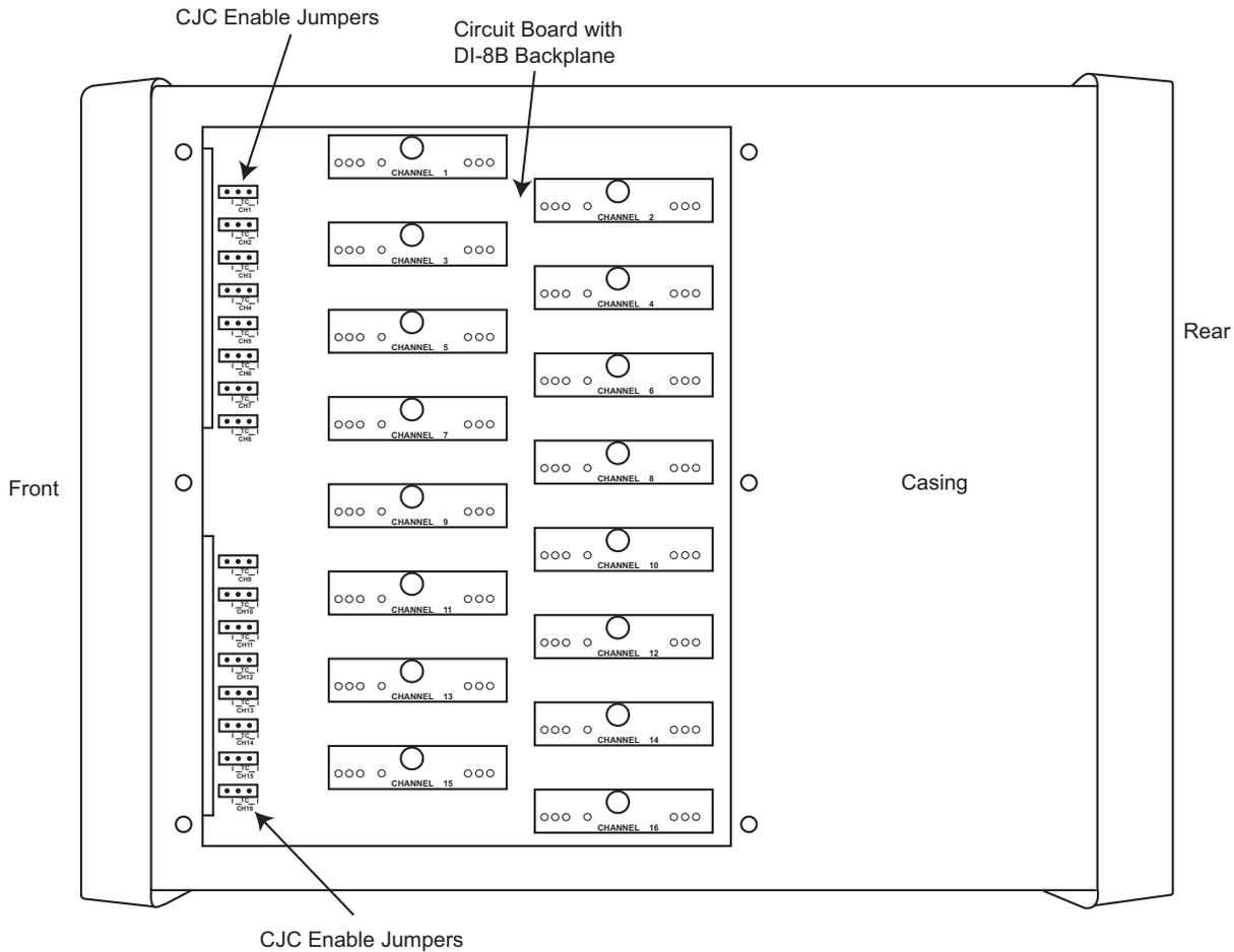
3. Each jumper is labelled on the circuit board as “TC CH#” where # is the channel number. Jumpers are installed on the circuit board in the “off” position. Move the jumper to the “TC” pins for each channel using a Thermocouple module. **Note:** If you are not using a Thermocouple Input Module on that channel be sure the jumper is disabled (in the “off” position) because this will affect the input signal.
