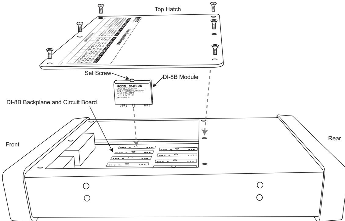
4. Using an erasable pencil write the module number of each DI-8B module installed on the sticker located on the top hatch to indicate which module is installed at each channel position.
