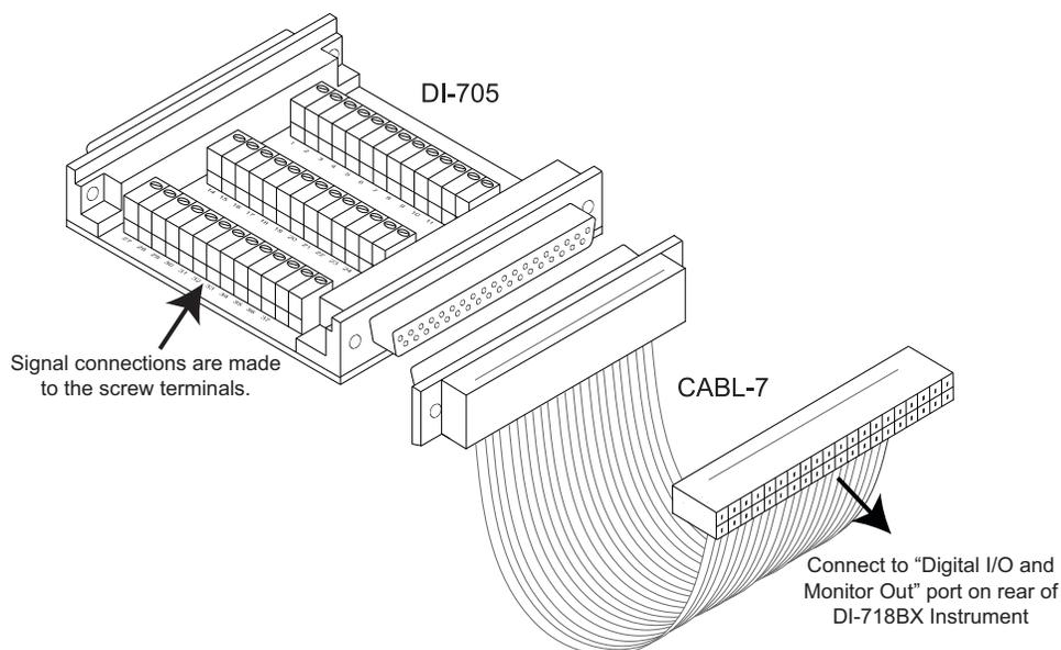
The Digital I/O may be enabled as Channel 17. **Note:** *The Digital I/O is not available in stand-alone mode — Except for Remote Start/Stop (DI/O0) and Remote Event (DI/O1).* Use the table below for pinout of the DI-705 (screw terminal in **bold**).
