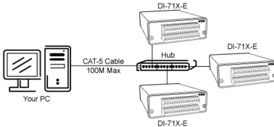
**Note:** For hubs that do not have an auto-switching sensor (usually older hubs) you must **not** use a crossover cable.
