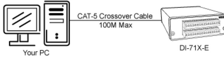
**Note:** When installing an Ethernet device directly connected to your PC you **MUST** use a crossover cable (provided).
