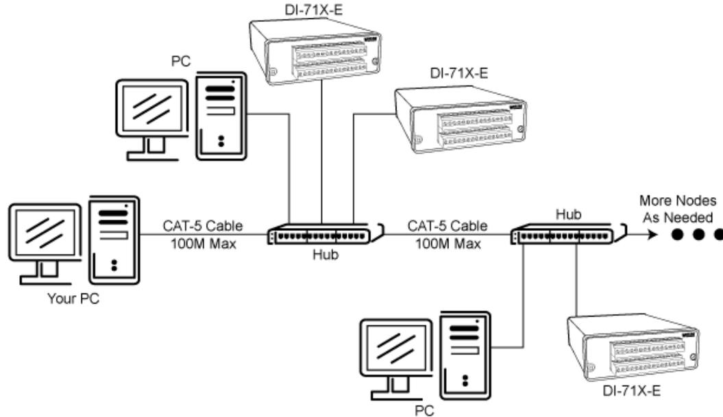
*Note:* In the illustration above, the Hubs could instead be routers with DHCP turned off (i.e., a static IP assigned network). Contact your system administrator for details about your network.
