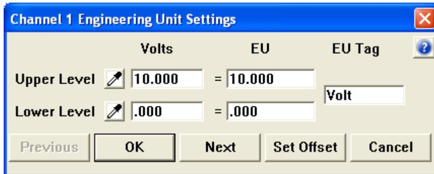
Enter the appropriate information in the available text boxes. For example, if using a DI-8B47K-05, the Input is 0°C to +500°C and the Output is 0V to +5V. Enter 5 in the Upper Level text box under Volts and 500 in the Upper Level text box under EU (5 volts = 500 degrees C). The Lower level text boxes should be 0 for both (0 volts = 0 degrees C). Enter the appropriate EU tag (here degrees C) Press OK to save the settings..
