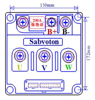
The controller installation should take consider of the heat dissipation and ventilation to avoid water spatter. and the wire connection instruction is as below,
