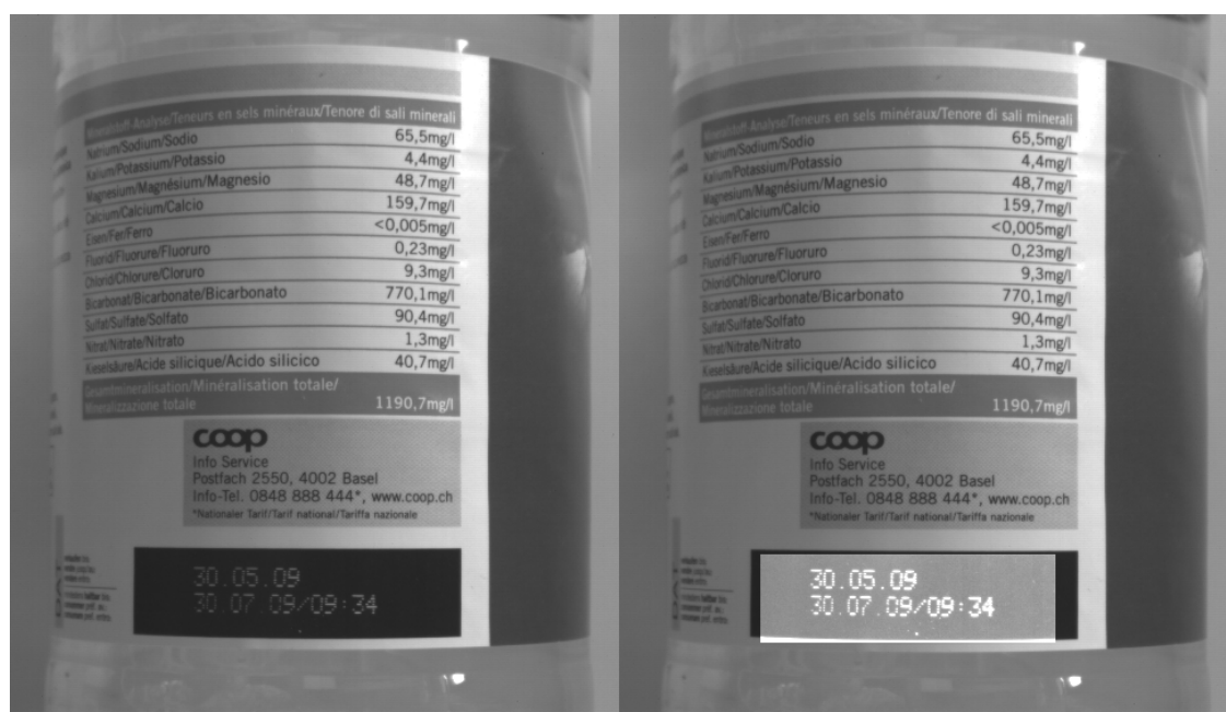
Figure 4.45: Region-LUT example with camera image; left: original image; right: gain 4 region in the area of the date print of the bottle
