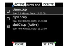
Multiple files can be selected. All checked files will be shown on graphics page and used in near mode calculation, when waypoint is of proper type (airport or outlanding place). However, only one file can be the active file. Active file is used for task creation.
