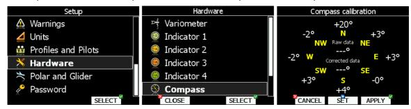
1. Orientate the glider to 360°. N label will be automatically focused
