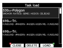
Total task distance, task description and task points are shown for each task stored. Select desired task rotating bottom-right knob and press LOAD. Task will be loaded into active task and task edit dialog will be opened.
