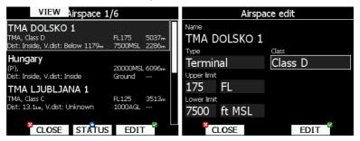
Pressing VIEW button, list will toggle views. When STATUS button is pressed status of selected airspace zone will toggle from **OFF always**, **OFF today**, **OFF hh:mm** and enabled. If EDIT button is pressed, new dialog will open, where you can modify properties for selected zone. See chapter 5.1.5.3 for more details.
