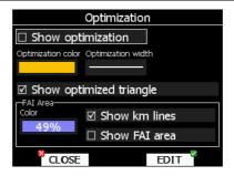
Check **show optimization** item to enable display of optimized track. Optimization color and width defines color and width for these lines.
