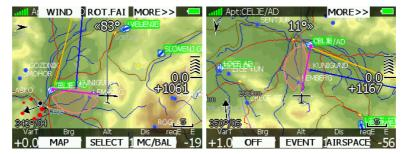
Press MORE>> button to see more options. If remote stick is available, behavior is slightly different. When check button is pressed on remote stick a menu will appear, instead of button functions.
