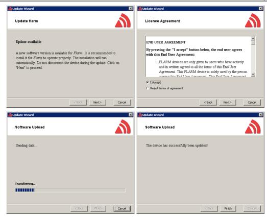
In case that Flarm stops working and update is not possible over described procedure with password 42000, use following recover procedure. In Flarm tool choose Recover and follow instructions. On LX8000 enter password 41000
