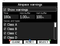
Airspace warnings are the most complex ones. Airspace warning is activated by two triggers: First warning (orange) will be given when a projected position of flight for period, which is defined in Time item, is computed to cross airspace zone.
