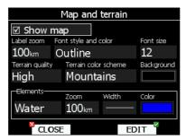
Check **Show map** item to enable map displays in navigational pages. If item is unchecked no map will be displayed. The **zoom** defines up to which scale of zoom city names are visible. 100km means the whole width of the screen represents 100km. The user can also modify size, font style and color by **Font style and color** item. Use left-bottom knob to modify color and right-bottom knob to modify style.
