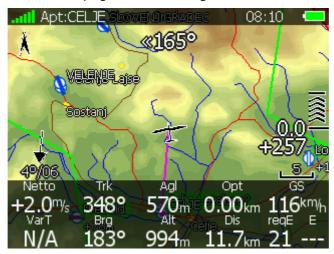
Current netto vertical speed, current track, height above ground, optimized distance and current groundspeed.
