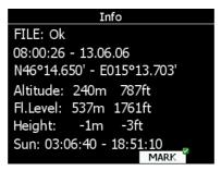
If you press MARK button, new waypoint will be created with current latitude and longitude and elevation based on terrain database. Waypoint name is generated from current date and time.
