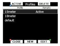
Use this dialog to add new profile, delete profile, change name for existing profile and activate. Active profile is profile which is currently being used. Press EDIT button and Edit profile dialog will open.
