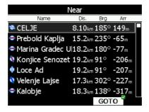
Select preferred landable place with bottom-right knob and press GOTO button. It will automatically change to airport mode and navigation will commence to selected point. Duplicates are automatically removed. If target with nearly same latitude and longitude is found in LX navigation's Airports database and user waypoint file, user waypoint file will be displayed.
