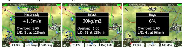
Use bottom-right knob to modify MacCready setting. In middle button there is a suggestion for MacCready setting, which is based on last four thermals. Additionally to selected MacCready value an overload factor is also shown and calculated glide ratio with corresponding speed.
