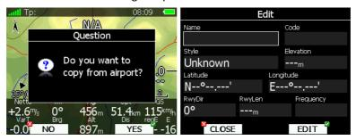
Minimum data that must be entered is name, latitude and longitude. Press CLOSE button to finish editing waypoint properties. New waypoint is added to active waypoint file.
