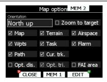
If Zoom to target check is selected, zoom will be automatically adjusted, so that target point is always visible. Maximum zoom is 200km and minimum zoom is 1km. Next checkboxes will turn on or off following items:
