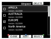
Select required airspace and press SELECT. If a checkmark is shown in front of airspace item, this airspace file will be shown in graphics and used for proximity calculation, when enabled.
