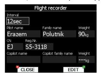
Select recording interval, enter pilot name. Pilot weight is important if ballast is given in kilograms of water. (See chapter 5.1.11). If LX8000 is used in double seater the name of copilot can also be entered.
