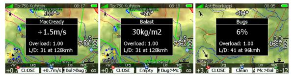
Use bottom-right knob to modify MacCready setting. See chapter 5.5.5.2 for more details It is also highly recommended to check safety altitude setting. See chapter 5.1.1 to find out how to setup safety altitude.
