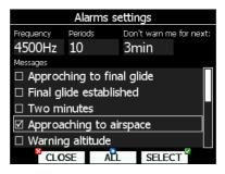
Use page selector to iterate through checkbox list. Press **ALL** button to enable all options.
