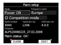
Flarm status message is normally OK. In case of any errors or warning, an error message will appear. User can change operation mode of Flarm unit, frequency and enables competition mode.
