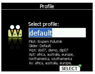
Turn bottom-right knob to select desired profile, if more then on profile is available. For selected profile pilot name, glider type, loaded waypoint files, loaded airports databases and loaded airspace databases are shown.
