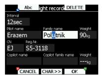
Press **CHAR>>** button to advance cursor to next position. Cursor can also be moved to next position using bottom-left knob. Rotate it clockwise to move forward.
