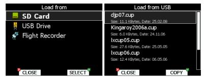
In next step, source of data must be selected. Flight recorder as source is not implemented yet. A dialog with list of all available files will be opened. Press COPY button to copy selected file to LX8000. LX8000 will accept following file formats:
