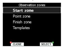
Each type of observation zone is defined with two angles, two radii and direction. Using these parameters enables the creation of any known zone geometry separately for start, turn point and finish.
