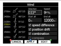
Wind profile is shown on left side of dialog. Yellow color altitude indicates our current altitude. Using bottom-left knob you can scroll wind layers up and down.
