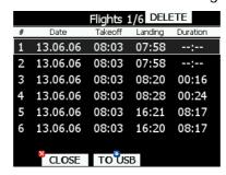
If SD card or USB stick is inserted in LX8000, flights can be copied to it, when appropriate button is pressed. Flights can be removed using DELETE button.
