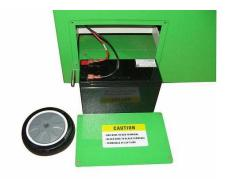
black wire to the black terminal. Care must be taken to ensure you put the battery terminals to the top left side when you insert the battery into the cage.
