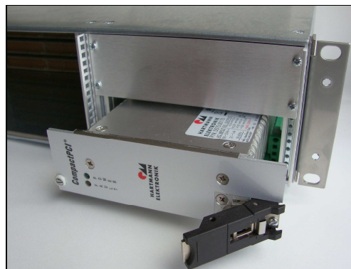
Figure 5-3 Replacing the Power Supply (sample: 2U version)
