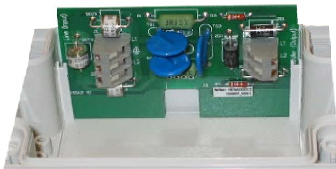
Serial Lightning Protection Module
