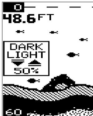
reach the maximum or minimum level, a tone sounds alerting you to the limits. The menu will clear automatically after a few seconds or you can press the PWR key to clear the screen.
