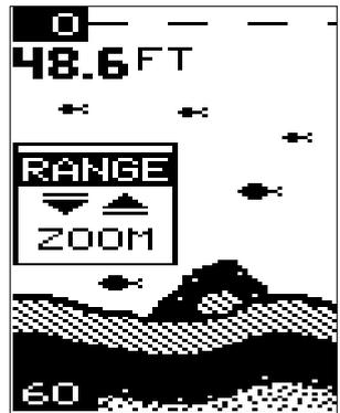
This is the zoom size menu. Zoom size is the distance between the upper limit and the lower limit. The upper limit shows at the top left corner of the screen. The lower limit is in the bottom left corner. For example, if the upper limit is 40 feet and the lower limit is 70 feet, the zoom window size is 30 feet. The word "TRACK" appears in this menu when you first activate the zoom as shown at right.
