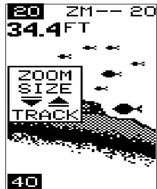
This means the unit is tracking the bottom in a zoom window, always keeping it on the display.
