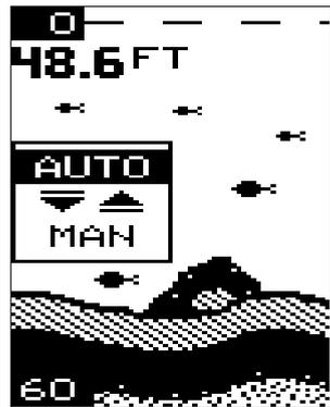
To turn the automatic feature off, press the menu key until the AUTO/MAN menu appears. Now press the down arrow key. This highlights the letters "MAN." The unit is now in the manual mode. Wait a few seconds and the menu will scroll off the screen's left side.
