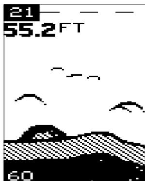
To change the lower limit, again make certain the unit is in the manual mode. Press a menu key until the "LOWER LIMIT" menu appears. Now press the down arrow key to increase the lower limit or the up arrow key to decrease it. When you have the limit set, wait a few seconds and the menu will scroll off the screen's left side. Pressing the PWR/CLEAR key also clears it.
