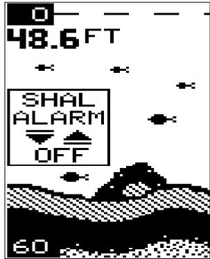
Press the up arrow key to silence the alarm. This will turn the alarm sound off until the shallow alarm is triggered again.
