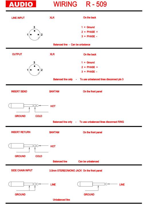
FIG. 2 External connections
