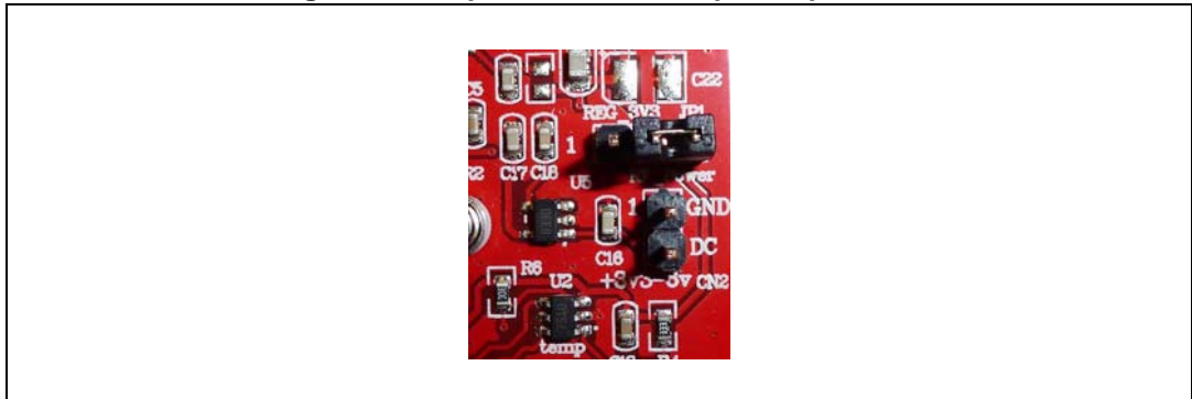
Figure 4. Jumper JP1 set in RF power position
