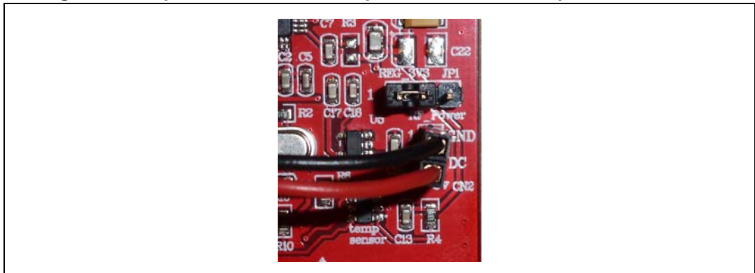
Figure 5. Jumper JP1 in “REG_3V3” position and external power connection
