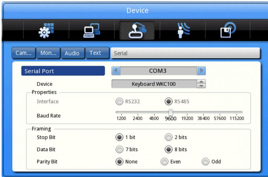
The Keyboard is already configured under DVR mode. Motordome cameras that are connected to the DVR and configured in the DVR can be controlled by the keyboard, too.
