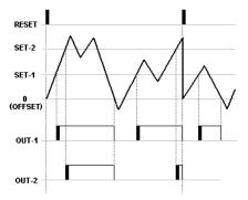
When count value rises above the level of the SET-1, OUT-1 is active and rises above level of the SET-2, OUT-2 is active. TOUT terms while selected HOLD, there is no outputs even to count value falls bottom level of SET values. Outputs will be reset when count value reaches zero (OFFSET), besides count value and outs will be reset when comes RESET.
