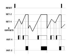
OUT-1 depends to OUT-2 and TOUT-2 should be selected as term. When count value rises above the level of the SET-1, OUT-1 is active and rises above level of the SET-2, OUT-2 is active. So count value will be fixed. Outputs and count value will be reset at the end of TOUT-2 period.
