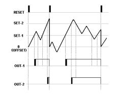
In this mode, when count value rises above the level of the SeT-1, OUT-1 is active and above the level of SET-2, OUT-2 is active. Relays will be active even goes down below the set values without RESET. Relays give outs during this time, if entered times for outs. Relays don't give outs until RESET.
