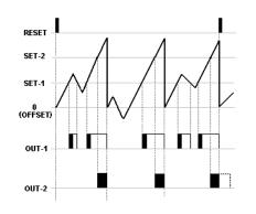
Output-4 continues counting after level of set-2 value. OUT-1 depends to OUT-2 and TOUT-2 should be selected as term. When count value rises above the level of the SET-1, OUT-1 is active and rises above level of the SET-2, OUT-2 is active. So count value will be fixed. Outputs and count value will be reset at the end of TOUT-2 period.
