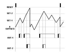
In this mode; when count value rises above the level of the SET-1, OUT-1 gives the out (so Relay-1 is ON). If TOUT-1 is selected (Time of Relay-1) HOLD, OUT-1 is active until count value falls bottom level of SET-1. When count value rises above the level of the SET-2, OUT-2 is give the out and If TOUT-2 is selected HOLD, OUT-2 is active until count value falls bottom level of SET-2. TOUT-1 and TOUT-2 are selected as term, OUT-1 and OUT-2 will active during this time.
