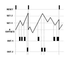
At this mode, TOUT-2 should be selected as term. OUT-1 is active during TOUT-1 period at count value exceeds the each value of the SET-1 and OUT-1 is inactive at the end of TOUT-2 period. Count value and outs will be reset when comes RESET.
