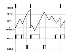
While count value is below level of Set-1, Out-1 is active and then Out-1 is inactive when on top of it. Out-2 is active when on top of SET-2 value and OUT-2 is inactive after reaching below the SET-2 value. Count value and outs will be reset when comes RESET.
