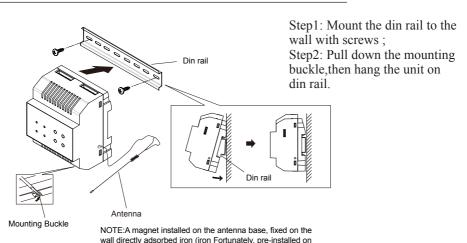
the wall) place. In addition, the antenna should be installed in the open place, there should be no obstructions around.
