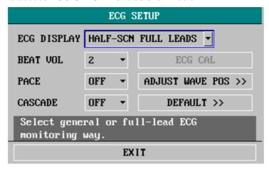
Figure 12-7 ECG SETUP menu
