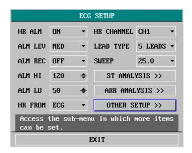
Figure 12-6 ECG SETUP menu
