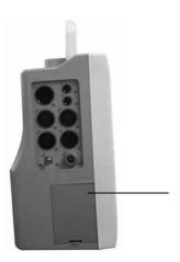
Figure 1-7 Battery Slot Cover
