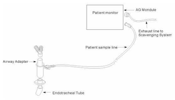
Figure 19-2 connection diagram for measuring AG gas
