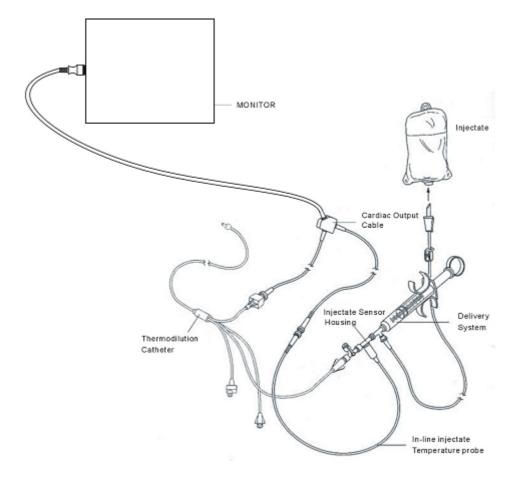
Figure 17-1 CO sensor connection
