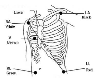
Figure 12-1 Electrode placement for 5-lead set
