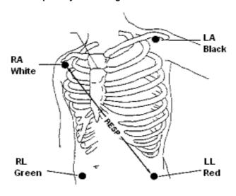
Figure 12-16 Electrodes placement (5-lead)
