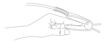
Figure 13-3 Mounting of the sensor
