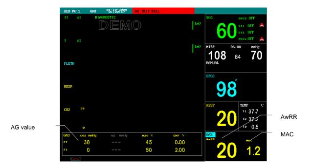
Figure 19-1 AG measurement display
