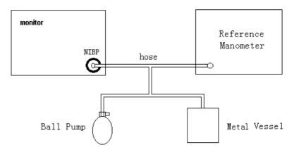
Figure 14-3 Diagram of NIBP calibration
