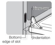
4. Push the hinge locks up against the front frame of the oven cavity to the locked position.
