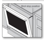
Leave the door open to the broil stop position. The door will stay open by itself, yet the proper temperature is maintained in the oven.
