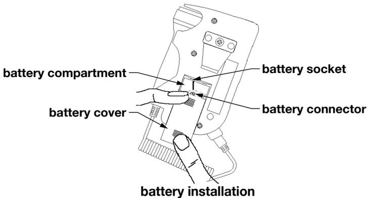
1. Open the battery compartment: Slide the battery cover in the direction of the arrow on the battery cover (see above picture).
