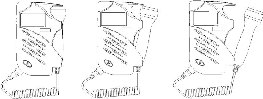
1. The probe is installed in Pocket Doppler probe frame (left picture above). Hold the Pocket Doppler main unit with one hand and hold the top of the probe with the other hand.
