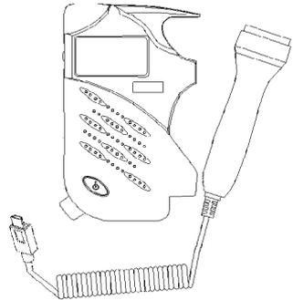
▲ **NOTICE: Place the unused probe in a secure location. When the Pocket Doppler is not used for a long time, store Doppler and probe in original packaging (see Maintenance/Storage section for proper storage conditions).**
