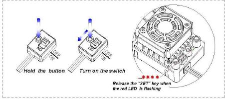
Note2: If you don't release the "SET" key as soon as the red LED begins to flash, the ESC will enter the program mode, in such a case, please switch off the ESC and re-calibrate the throttle range again from step A to step D.
