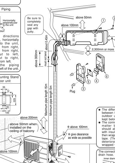
The difference in height between the indoor and outdoor unit should be kept below 5m.
