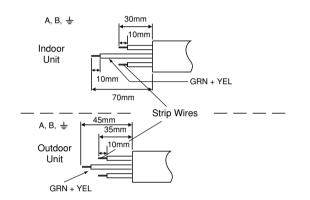
Detail of cutting the connecting cord
