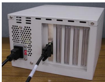
Figure 2.9. Plugging the power cable into the ECH-PE-CE2-F4A
