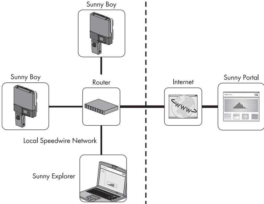
Figure 2: PV plant with a Speedwire network in star topology (example)
