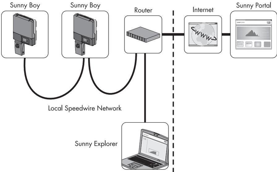
Figure 1: PV plant with a Speedwire network in linear topology (example)
