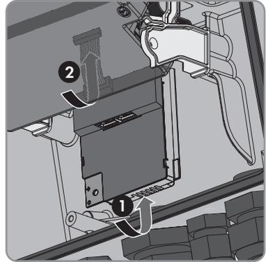
6. Fasten the Webconnect Data Module hand-tight with the hexagon socket screw.
